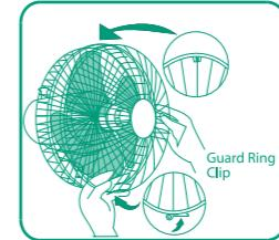
4. Hold the front guard with logo in upright position and attach it to the rear guard. Secure the two guards by fastening the clip.
