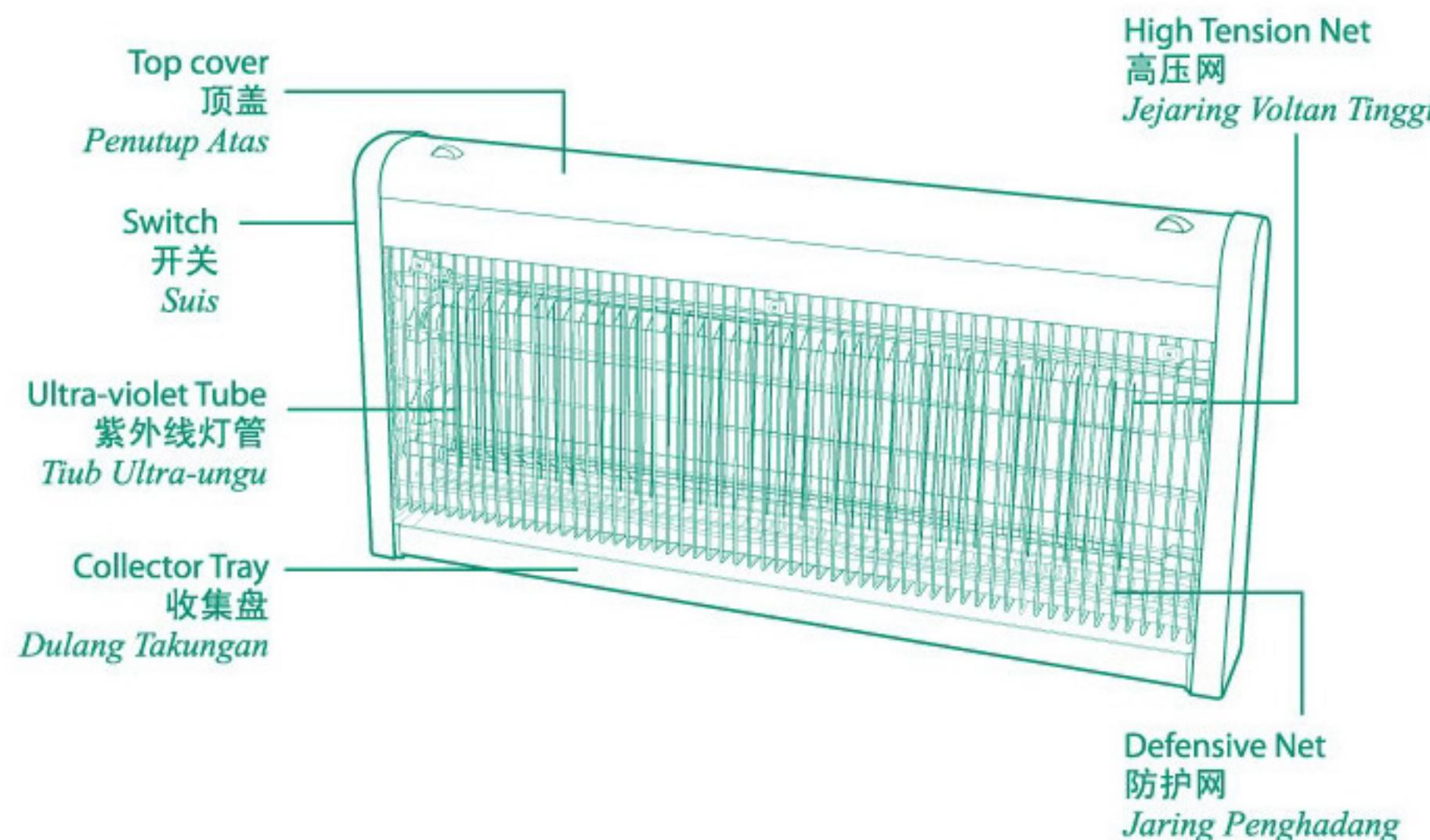
1. Do not touch the HIGH TENSION NET with hand or any electric conductor.
