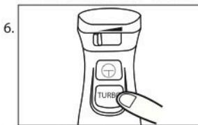
Press the Turbo Button for highest speed.
