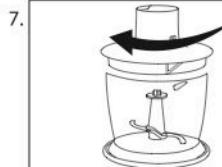
Attach the chopper lid by aligning the locks. Turn clockwise to complete locking process.
